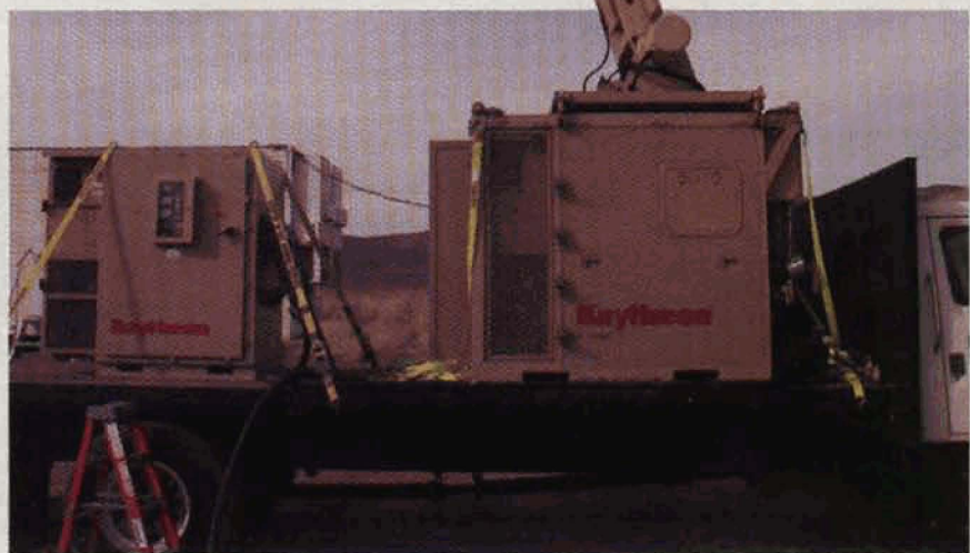
Silent Guardian is one of the first directed-energy weapons ready for deployment. Its millimeter-wave-beam heats water in the skin to the point of pain.
